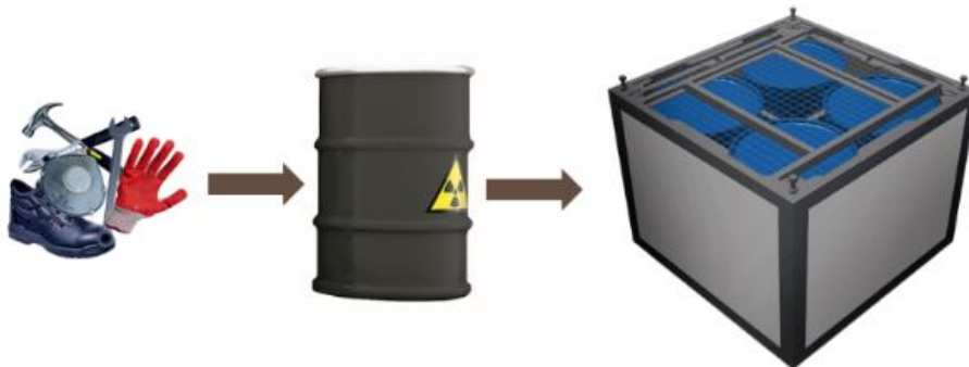
Figure 3.3.5-1. Compact waste package containing low- and intermediate-level radioactive waste, produced using a steel container
