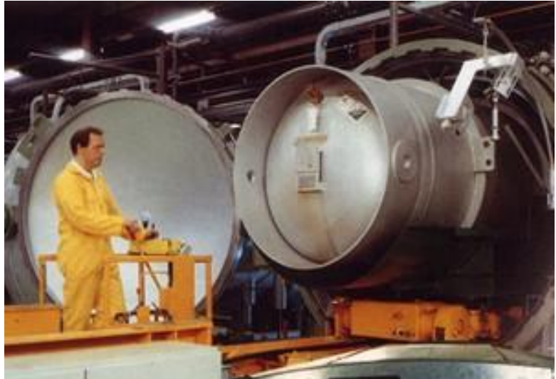
\text{UF}_6 tank in an enrichment plant
